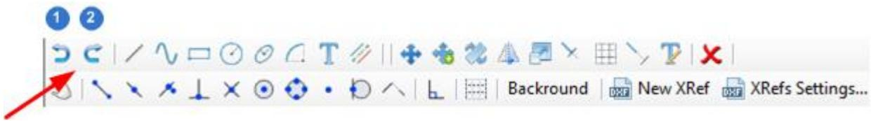
Drawing mode has its own local undo (1) redo (2) stack which is reset after leaving the drawing mode.
